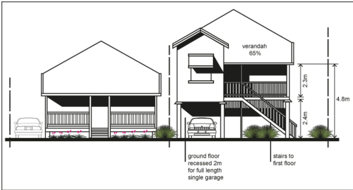
Figure a—Elements of typical elevation
